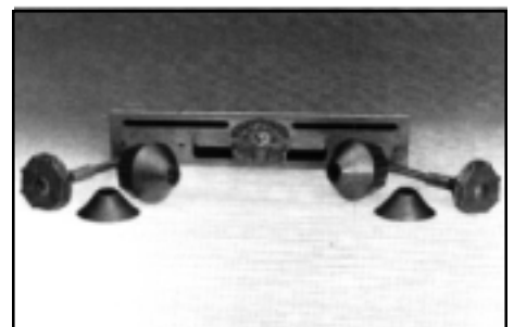
Bolt holes that are offset can be matched by setting the DSL at the desired offset angle prior to rotating the flange.
