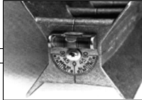
A built-in protractor provides easy, accurate measurement.
