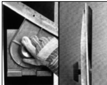
Angles can be easily locked in place by hand tightening the adjustment knob.
